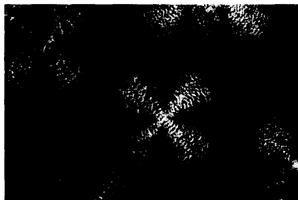
Figure 8 Optical micrographs (crossed polars) of PHB spherulites growing around an EPR liquid domain ( T_c = 115^\circ\text{C} ) for PHB-EPR 70/30 blend at different times, t : (a) t = 4 min; (b) t = 6 min; (c) t = 8 min; (d) t = 10 min
