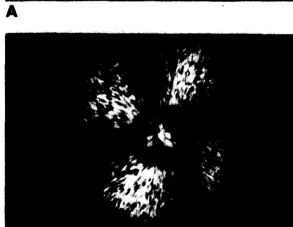
Figure 12 Optical micrographs (crossed polars) of growing PHB spherulite at T_c = 105^\circ\text{C} (A) and at T_c = 110^\circ\text{C} (B) for PHB-PVAc 50/50 blend
